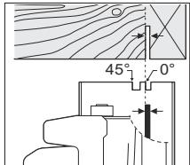
The  $0^\circ$  cutting mark indicates the position of the saw blade for right-angled cuts. The  $45^\circ$  cutting mark indicates the position of the saw blade for  $45^\circ$  cuts.
