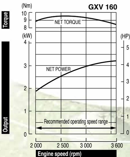
The power rating of the engine indicated in this document is the net power tested on a production engine for the engine model and measured in accordance with SAE J1349 at a specified rpm. Mass production engines may vary from this value. Actual power output for the engine installed in the final machine will vary depending on numerous factors, including the operating speed of the engine in application, environmental conditions, maintenance, and other variables.
