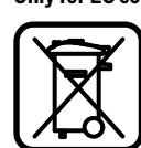
According to the European Directive 2012/19/EU for Waste Electrical and Electronic Equipment and its implementation into national right, power tools that are no longer usable must be collected separately and disposed of in an environmentally correct manner.
